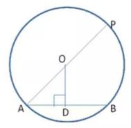
AD = DB = 1.6cm (Perpendicular from centre to a chord bisects the chord) In right  $\triangle$  ODA, By Pythagoras theorem, OA<sup>2</sup> = OD<sup>2</sup> + AD<sup>2</sup> = 1.6<sup>2</sup> + 1.2<sup>2</sup> = 2.56 + 1.44
